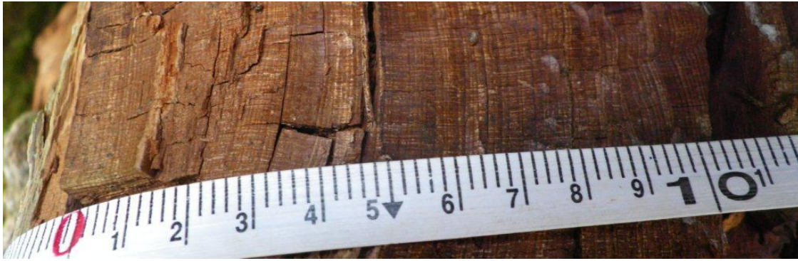
Sample A: Mean ring width 0.78mm over 10 cm. (Yew 1 outer bole section fell 2005).
